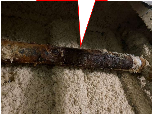
Lateral drain lines that had active leaks were found on every floor
